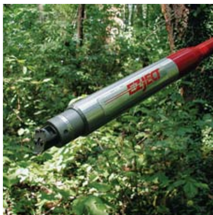
11. The E-Z Ject lance injects capsules into stems.
