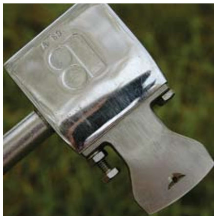
11. The E-Z Ject lance injects capsules into stems.
