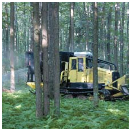
30. KMC track skidder with air-blast sprayer treating understory vegetation.
